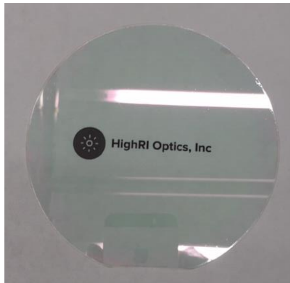
Spin-Coated Film of HighRI-Nano1.93 (600 nm thickness) on a 4-inch wafer.
